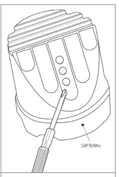
Remove the stainless steel mesh filter for cleaning by gently pushing a narrow object through the holes on the bottom of the metal barrel.
